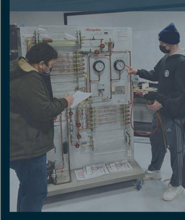
Photo above: International Union of Operating Engineers Local 30 - Union apprentices working with a heat pump trainer. The heat pump trainer is focused on new HVAC technology applicable to almost any facility where the power source is electricity rather than fossil fuels.
